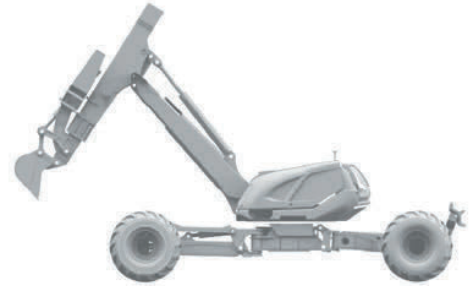
5 Elevation view of the autonomous walking excavator.
